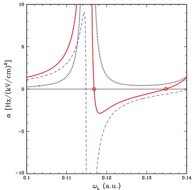
FIG. 3 (color online). Differential polarizability for Al  $\mu\text{Magic}$  clock in the  $\mathbf{B} \parallel \hat{k}$  geometry as a function of the lattice laser frequency. Dotted line, contribution from the scalar term; dashed line, contribution from the tensor term; solid line, total differential polarizability. Total clock shift vanishes at two values of the laser frequency.
