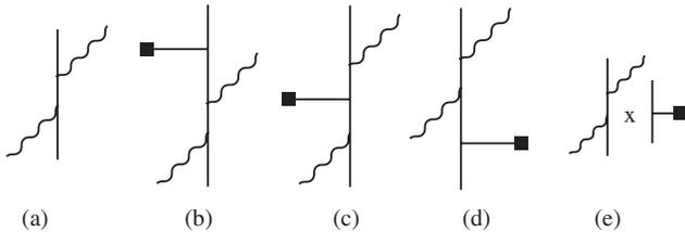
FIG. 1. Contributions to the dynamic polarizability  $\alpha(\omega)$ . Interactions with the laser photons are shown with wavy lines and hyperfine interaction with the capped solid line. (a) Second-order  $\alpha^{(2)}(\omega)$ . Contributions (b)–(e) are the third-order contributions to polarizabilities’ (b) top, (c) center, (d) bottom, and (e) normalization diagrams.
