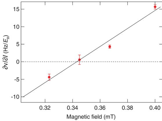
FIG. 4 (color). Sensitivity of the transition frequency to the lattice laser intensity ( $\partial\nu/\partial I$ ), as a function of the bias magnetic field, at  $\lambda = 806$  nm. At  $B = 0.343(3)$  mT (i.e.,  $20 \mu\text{T}$  away from the magic field),  $\partial\nu/\partial I = 0$ , and the transition becomes insensitive, at first order, to fluctuations of the light intensity, with a residual field sensitivity  $\partial\nu/\partial B$  of  $1.7 \text{ Hz}/\mu\text{T}$ .
