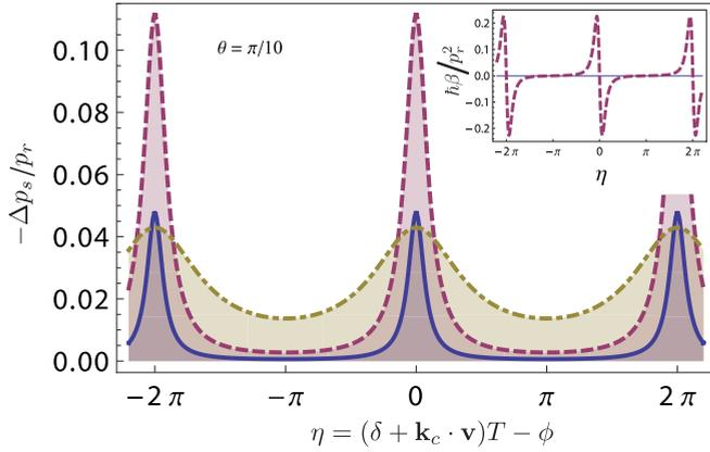
FIG. 3. (Color online) Frequency dependence of the fractional momentum for a pulse area  $\theta = \pi/10$ . The three curves differ by the values of the parameter  $\gamma T$  (solid curve,  $\gamma T = 0.1$ ; dashed,  $\gamma T = 0.447$ ; and dot-dashed,  $\gamma T = 2.5$ ). The spikes reflect the underlying frequency-comb teeth structure of the pulse train in the frequency domain. Inset: friction coefficient  $\beta$  as a function of phase for the dashed curve of the main graph.
