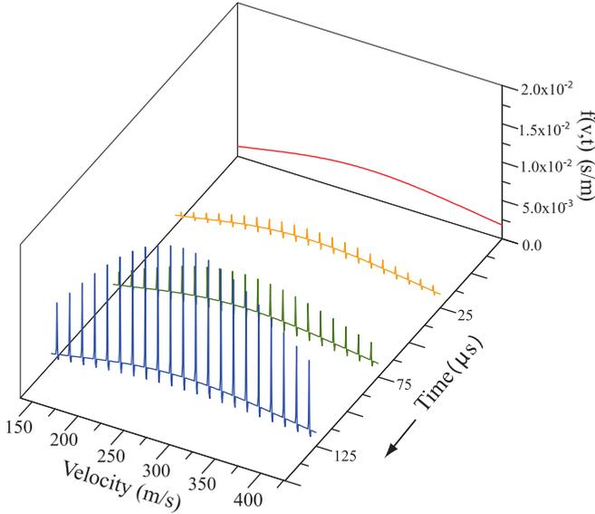
FIG. 4. (Color online) Time evolution of the velocity distribution for a thermal beam subjected to a coherent train of laser pulses. The pulse-to-pulse phase offset of the train is varied linearly in time as prescribed by Eq. (13). Atomic and pulse train parameters are  $\gamma T = 0.0026$ ,  $\theta = 0.0019$ . The optimal phase detuning is  $\bar{\eta} = 0.001$ . The characteristic initial temperature of the ensemble is 293 K.
