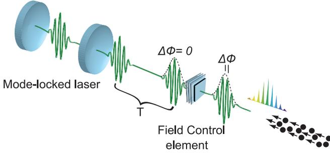
FIG. 1. (Color online) Schematic of a typical experimental setup. An atomic beam is slowed and cooled by a train of laser pulses. The phase and shape of pulses may be varied in time to attain optimal cooling.
