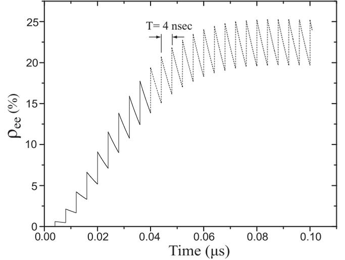
FIG. 2. Evolution of the excited-state population due to interaction with a train of laser pulses. The atom is initially in the ground state, and it is driven by a train of pulses separated by  $T = 4$  ns and of pulse area  $\theta = \pi/10$ . Radiative lifetime is 16 ns.
