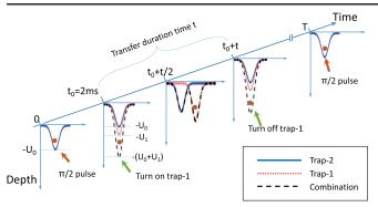
FIG. 4. Schematic illustration of the transfer process of a mobile qubit. An atom in a superposition state (the qubit) is initially confined in the static ODT (trap-two laser). It is then overlapped with the mobile ODT (trap-one laser). The qubit is extracted out by the mobile ODT and becomes a mobile qubit. The mobile qubit travels for a time interval t, and then it is returned to the static ODT.
