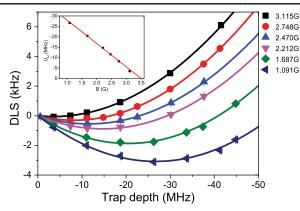
FIG. 2. DLS in the presence of hyperpolarizability. The DLS of a qubit in the circularly polarized trap-two laser is measured as a function of trap depths at various magnetic field strengths. The solid curves are fits to Eq. (1). The inset plots the minima  $U_M$  in the DLS curves as a function of magnetic field *B*. The light intensity of each minimum is chosen as the magic intensity at that *B*-field value.
