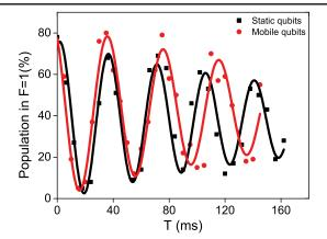
FIG. 5. Measured Ramsey signals for single static qubits (black squares) and single mobile qubits (red dots) at B = 3.115 G. Every point is an average over 100 experimental runs. The solid curves are fits to the damped sinusoidal function. The fitted values of coherence times  $\tau$  of static qubits and mobile qubits are 206  $\pm$  69 ms and 205  $\pm$  74 ms, respectively.
