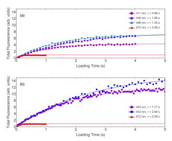
FIG. 5. Measured Ca MOT loading curves for (a) the  ${}^1P_1$  and (b) the  ${}^1P_1$  repump transitions, MOT fluorescence is plotted as a function of time elapsed after the cooling lasers are turned on; curves fitted to  $N(t) = R\tau(1 - e^{-t/\tau})$  are shown alongside the data.
