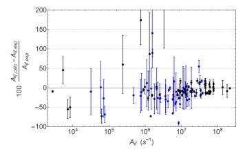
FIG. 1. Comparison of the calculated CI + MBPT transition rates with 111 available experimental data. Transitions involving a state with orbital angular momentum  $l \ge 3$  or principal quantum number  $n \ge 6$  are shown in blue. All other transitions are shown in black. Error bars correspond to the experimental error.
