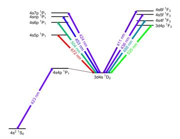
FIG. 3. Simplified calcium electronic level structure showing the eight repumping transitions considered here. All transitions except those at 504 and 535 nm have been studied experimentally. The overall best Ca MOT performance is found when pumping to a highly configuration-mixed state, labeled 4snp  $^1P_1$ , using the 453-nm 4snp  $^1P_1 \leftarrow 3d4s$   $^1D_2$  transition.
