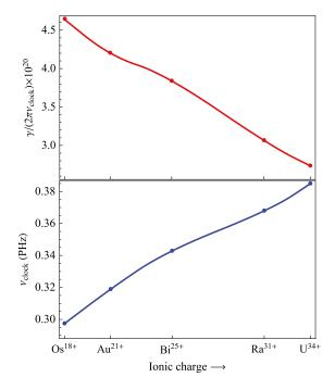
FIG. 1 (color online). Systematic trend of basic clock properties for the  $[Pd]4f^{12}$  isoelectronic sequence. Clock frequencies (lower panel) and the ratios of radiative linewidth to the clock frequency (upper panel) are shown as a function of ionic charge. Clock frequencies lie in laser-accessible near-infrared and optical domains, while the narrow transition width assures high quality factor.
