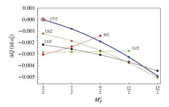
FIG. 3 (color online). Differential quadrupole moment  $\Delta Q$  as a function of magnetic quantum number of the excited clock level for  $^{209} \text{Bi}^{25+}$ . Different curves are labeled by values of the total angular momentum of the excited state F. The ground state hyperfine component remains fixed  $|F_g=13/2, M_g=9/2\rangle$ . The minimal value of  $\Delta Q$  is encircled; it is attained for the  $|F_e=17/2, M_e=\pm 5/2\rangle$  magic state.
