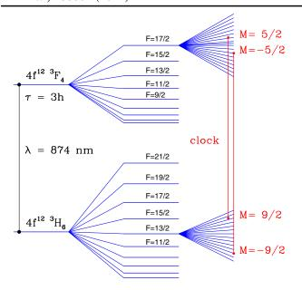
FIG. 2 (color online). Proposed virtual clock transitions in <sup>209</sup>Bi<sup>25+</sup> highly charged ion. Averaging over the two indicated transition frequencies removes the first-order Zeeman shift. Specific choice of hyperfine components and magnetic substates minimizes shifts due to couplings to gradients of the trapping electric field.
