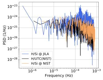
FIG. S7. Maser model and link noise contribution. Power spectral density of fractional fluctuations of the  $f_H/f_c$  ratio as measured at JILA (blue) compared to NIST (orange). The absence of a peak at  $2 \times 10^{-4}$  Hz in the NIST comparison shows this peak arises due to link noise. The maser comparison with UTC (black) further reinforces this conclusion.
